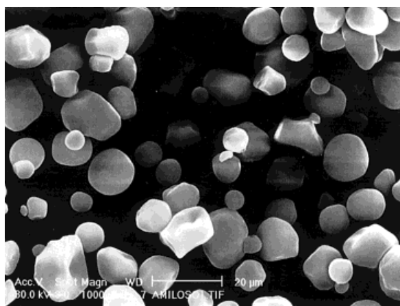
Figure 2 SEM micrograph of the starch amylo maize powder.
